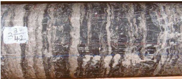
图1 XL101井大安寨段灰黑色炭质页岩 Fig. 1 Grey dark carbonaceous shale in the Da'anzhai Member of Well XL101
